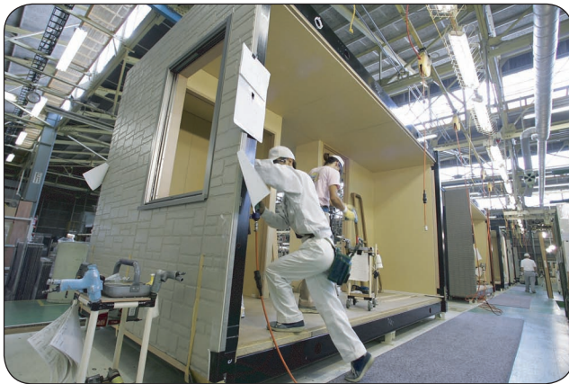
Housing units move on the production line as employees of Toyota Motor Corporation work during the installation process at the company’s Kasugai Housing Works, one of the plants of Toyota home-brand houses on Kasugai, Aichi Prefecture, Japan. Toyota entered the housing industry 30 years ago applying the plant technology and experience it gained through producing cars.
